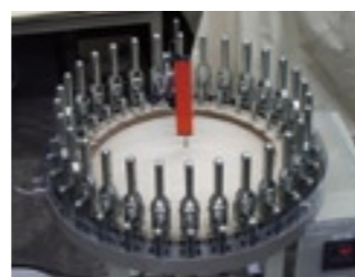
Creep test by hydraulic control method
